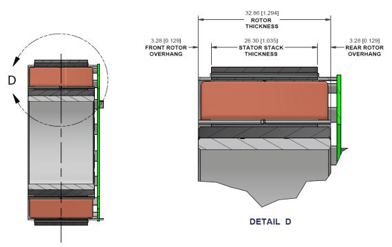
Figure 8. Detail view of Rotor to Stator Alignment on Sensor-less Motor version
