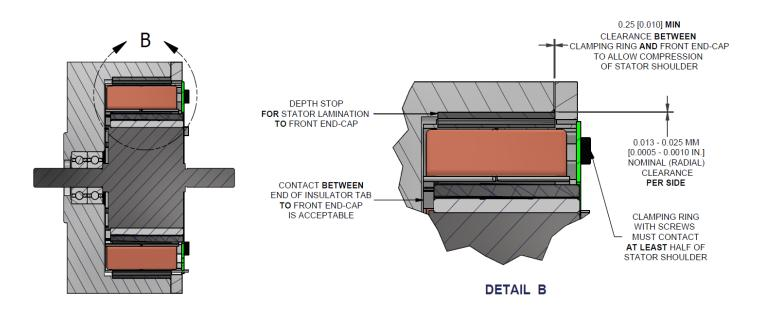
Figure 5. Detail view of Stator Axial Clamping to Housing Assembly
