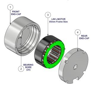
Figure 2. Exploded view of Stator to Housing Assembly with Bonding Method
