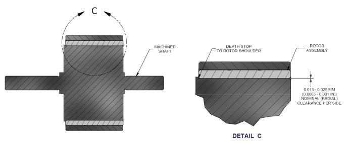
Figure 7. Detail view of Rotor Shaft Assembly
